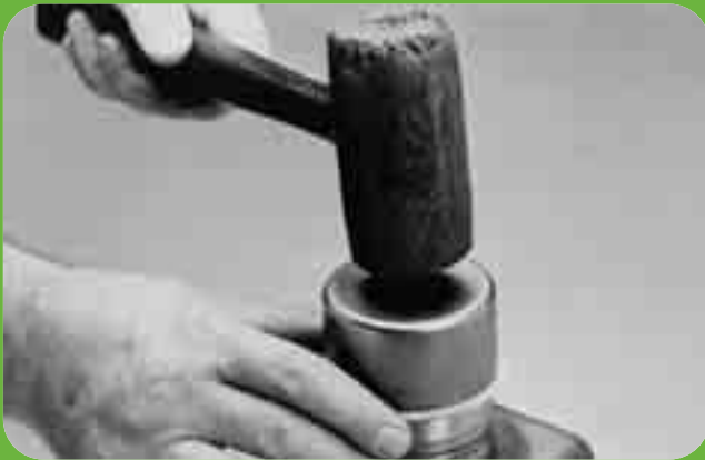
7 Tap tool to install Sleeve over shaft.
