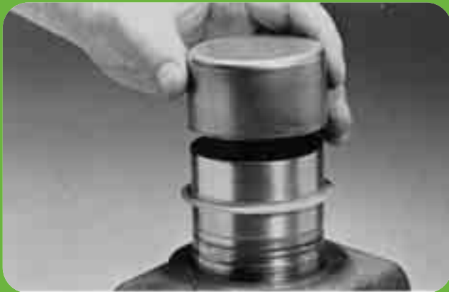
6 Place installation tool over Speedi-Sleeve®.
