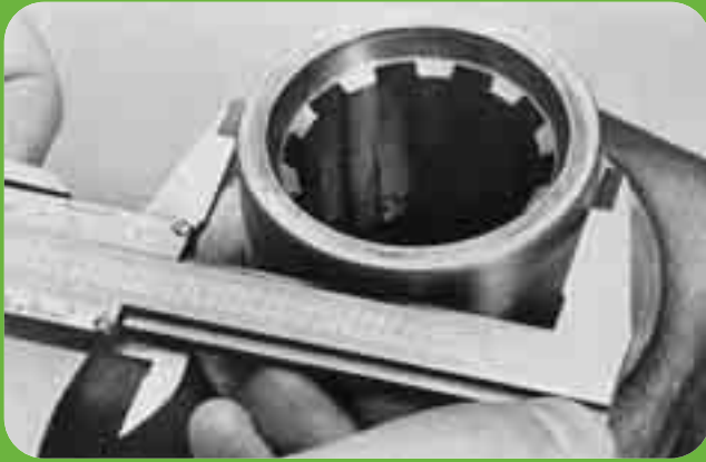
2 Measure shaft diameter in three places.
